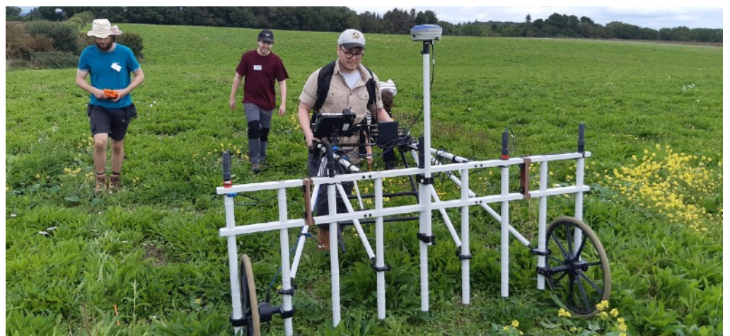
FIGURE 1: GEOPHYSICAL SURVEY USING A CART-BASED MAGNETOMETER.
